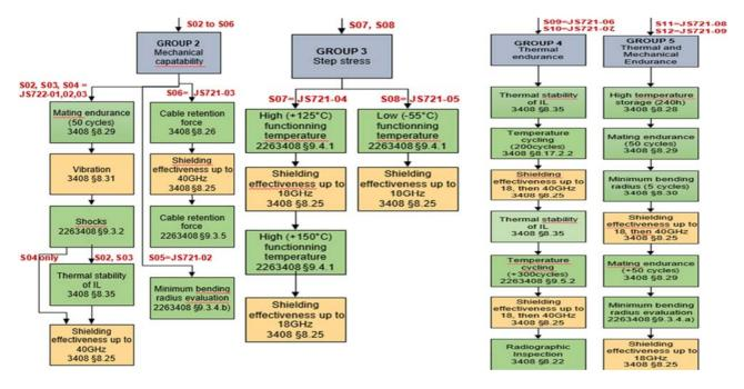
All tests performed at Axon', except vibrations, shocks and shielding effectiveness measurement up to 40GHz which are done at Radiall.
